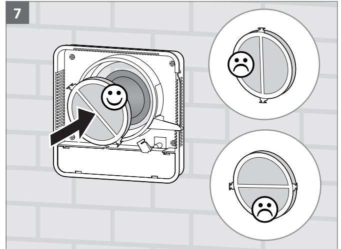
Slide the filter into the casing as far as the wall
